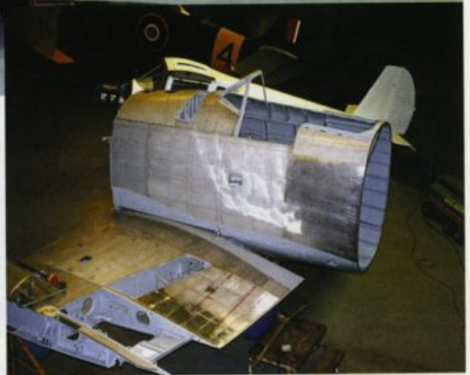
The battered center section of TG114 was rebuilt into pristine condition. (Sanders Family)
